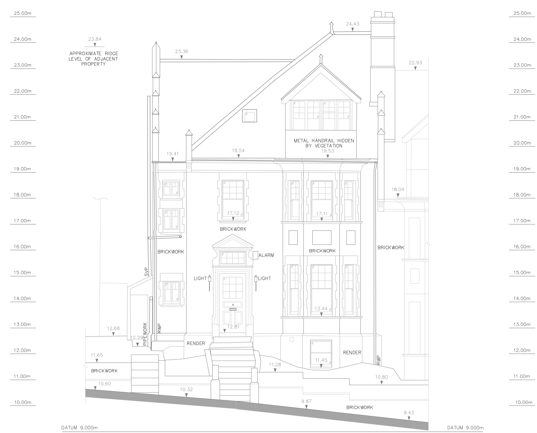
EXISTING FRONT ELEVATION
